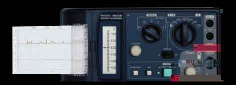
For voltage measurements, the display can be expanded from 25% to -35% around the center of the range. The center value can be changed in steps that are -10% of the range, which is convenient when it is presessing to adjust the management.
